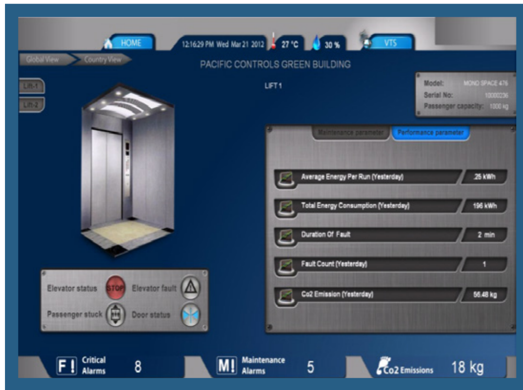
Example dashboard for Elevator Management
